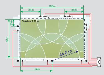
Irrigation sequence: 7 irrigation sections Flow rate: 1 sprinkler at the sidelines Q=39 m<sup>3</sup>/h Q=39 m<sup>3</sup>/h Max. flow rate per irrigation section Operating pressure: Pressure at the sprinkler nozzle H= 8,0 bar Required flow pressure at the connecting H=10,0 bar terminal for a water intake of 20 m3/h **Precipitation:** Average precipitation density 7,0 mm/h No. of sprinklers: Full and part circle sprinkler VP2M - 18 mm 7 pcs
