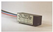
A bi-directional decoder is required with the possibility to return information back to the system contrary to a conventional decoder which can only receive information from the control unit.
