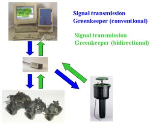
The Greenkeeper Control system compares the planned and actual value. In case of divergence immediately a dialog field with ERORR STATUS appears with the replied error.
