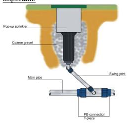
• Flush the pipes proper before installation of the sprinklers
